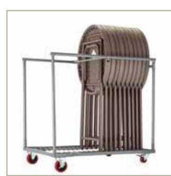
**Locking bar which moves along the side rails to fix the tables in position even at half load. The bar revolves around one of the rails to allow access to the back of the trolley, making it easier to load.**
